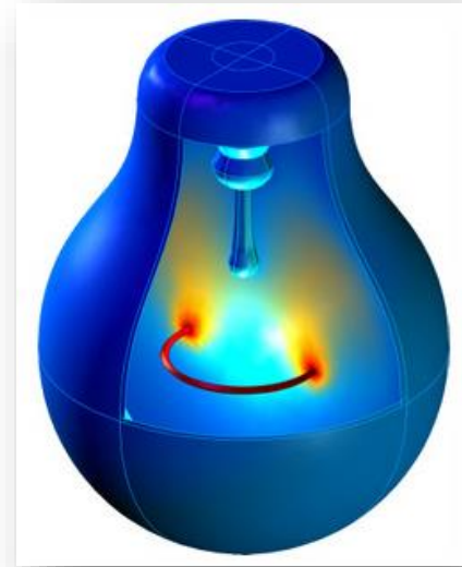
Temperature distribution in a light bulb generated by the radiating filament
