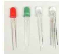
Figure 2.1: Discrete LEDs; from left to standard red and green, high-efficiency in various colors, and RGB.
