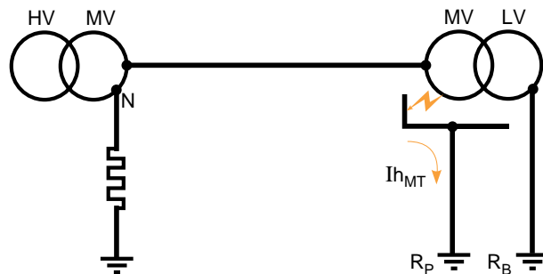
fig. 9a: if R_p and R_B are connected, the fault current causes the potential of the LV network to rise with respect to the earth.
