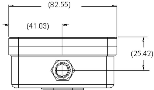
**Figure 12 Antenna Connector**
