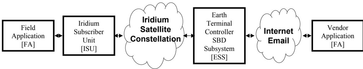
**Figure 1 Short Burst Data Architecture.**
