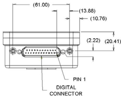
**Figure 11 Multi-Interface Connector**
