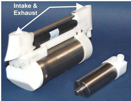
1. Install the data I/O cable, pump, and optional DO sensor cable on the GPCTD:
