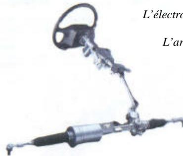
Figure 6 : direction assistée " coaxiale "
