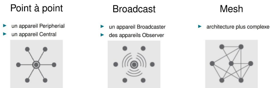
Figure 5 : Topologies de communication
