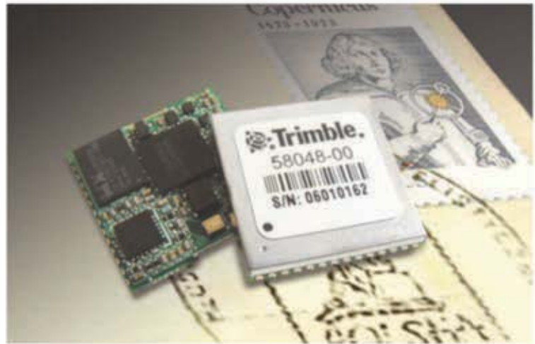
The Copernicus GPS Surface Mount Module and Shield
