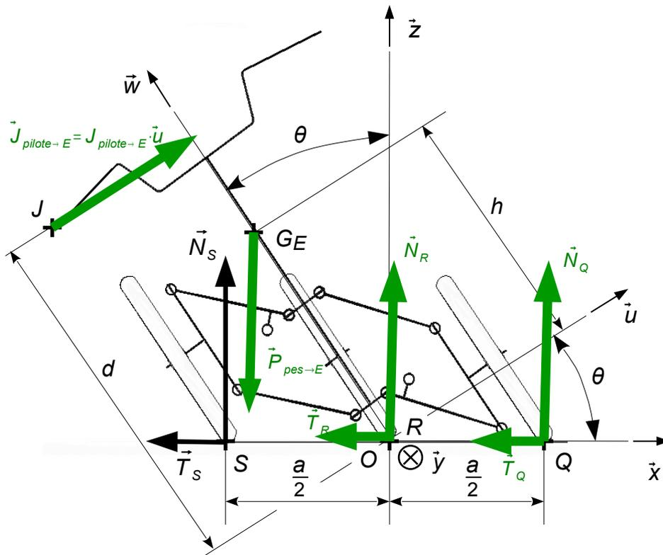
$$J(\text{pilote} \rightarrow E) \times d + N_s \times \frac{a}{2} - P(\text{pes} \rightarrow E) \times h \times \sin \theta - N_Q \times \frac{a}{2} = 0$$
