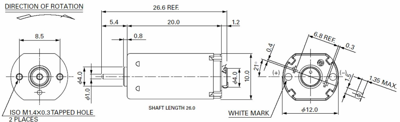
Usable machine screw length 1.3 max. from motor mounting surface.
