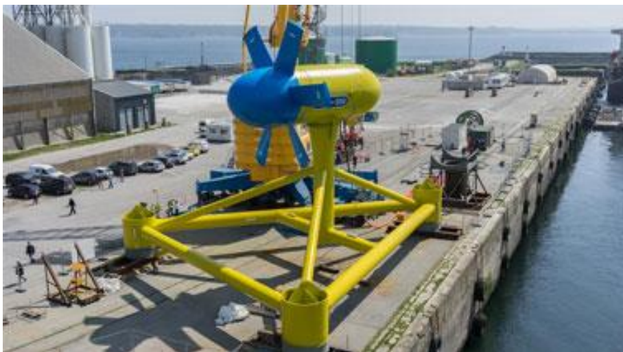
Figure 1 Hydrolienne Sabella D10.
