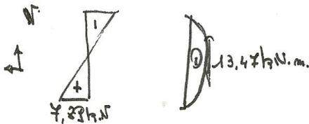
$$V_{pl,2,Rd} = \frac{1530 \times 245 \cdot 10^{-3}}{\sqrt{3 \times 1}} = 252,4 \text{ kN}$$
