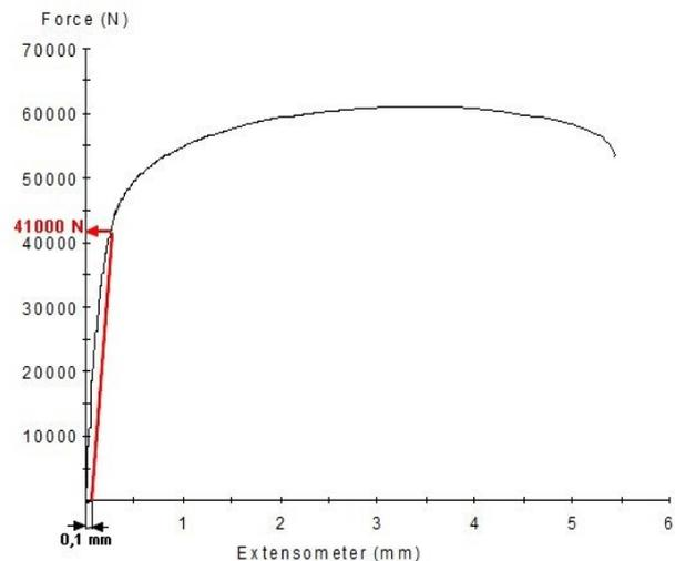
$$\text{Puis } R_{p0,2} = \frac{F_{p0,2}}{S_0} \Rightarrow R_{p0,2} = \frac{41000}{78,5}$$
