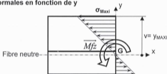
$$\sigma_{\text{Maxi}} = \frac{\left\| \frac{Mfz}{IGz} \right\|}{\left( \frac{v}{v} \right)} \text{ en MPa}$$
