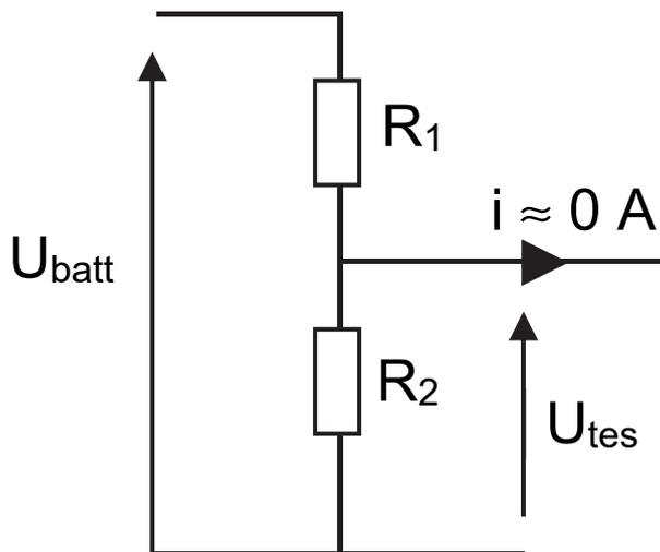
$$U_{test} = \frac{U_{batt} \times R_2}{(R_1 + R_2)}$$
