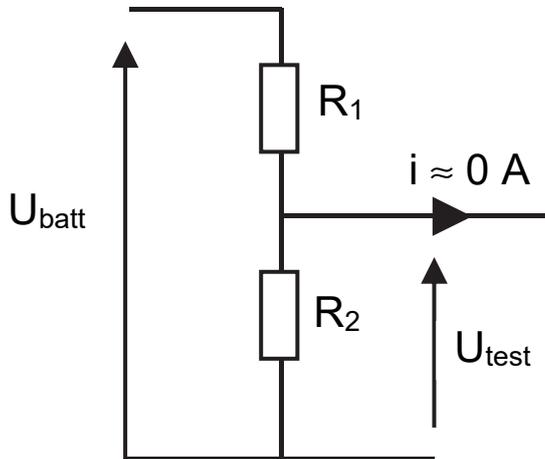
$$U_{test} = \frac{U_{batt} \times R_2}{(R_1 + R_2)}$$
