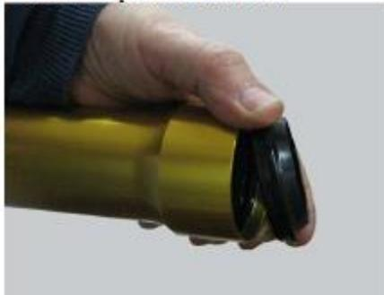
Déposer le circlip.
