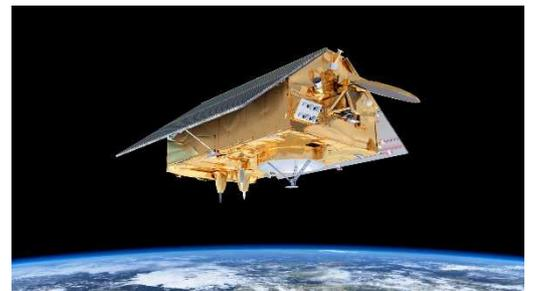
Figure 1. Satellite Jason-CS/Sentinel-6
