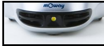
Image 10. Location of Obstacle Sensor
